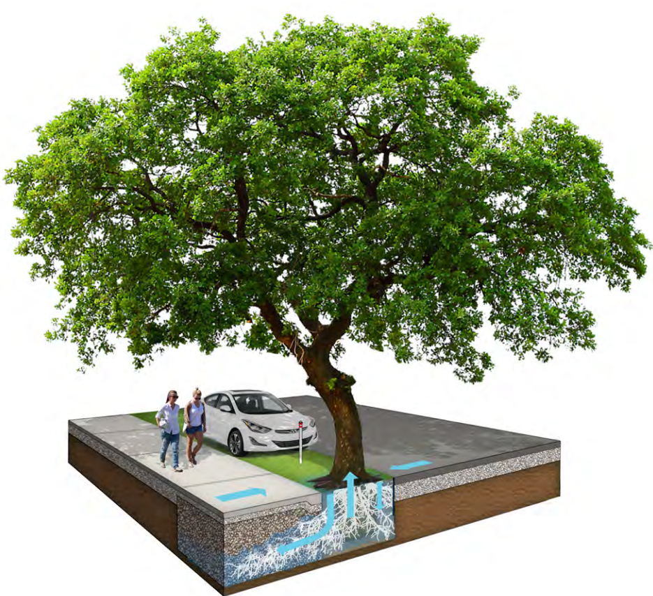
Large species tree in small swale - with CU-Structural Soil
