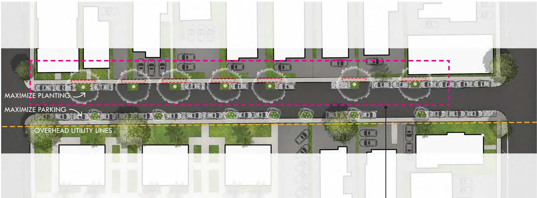
Large species tree with Structural Soil and porous pavement with a Tree Protection pole where cars can park adjacent on the side of the street with no overhead utilities.
