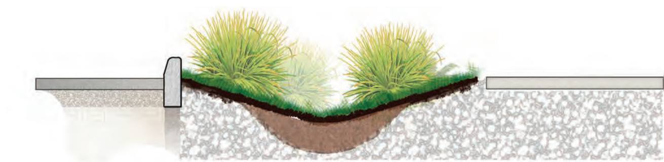
Figure 1: Rain Garden Section
