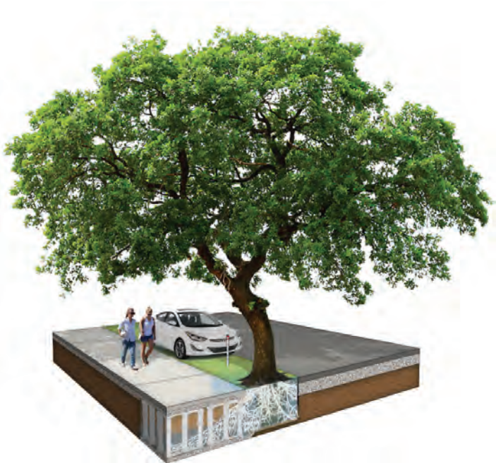
Large Tree Planted with Soil Cells beneath sidewalk
