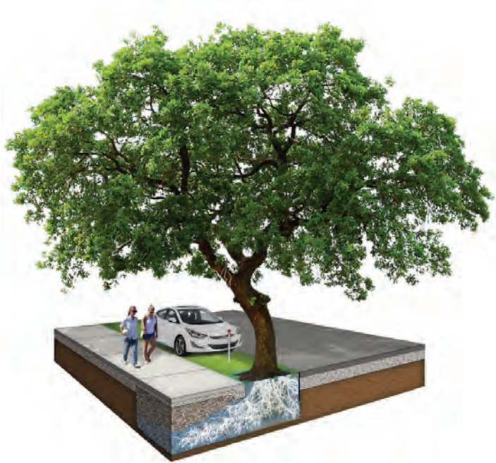
Large Tree Planted with Structural Soil beneath sidewalk
