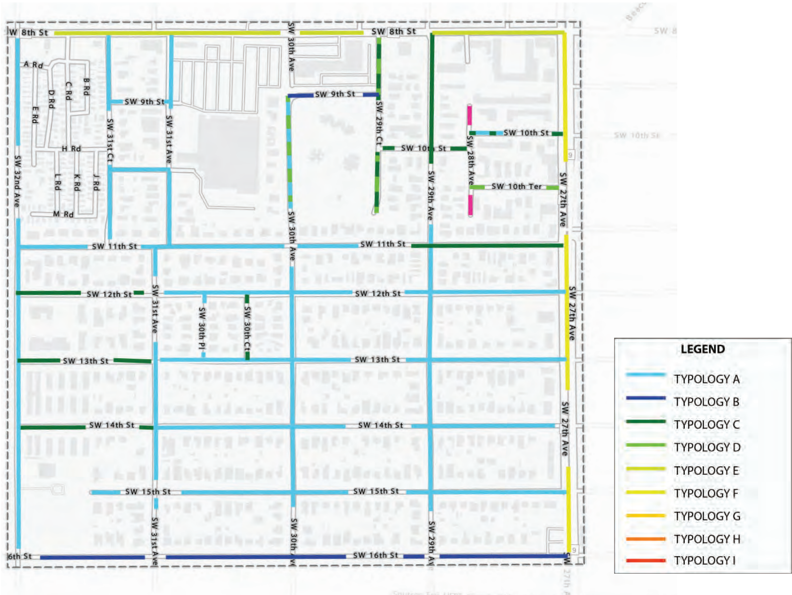
Figure 22. Parkdale North Street Typology Distribution
