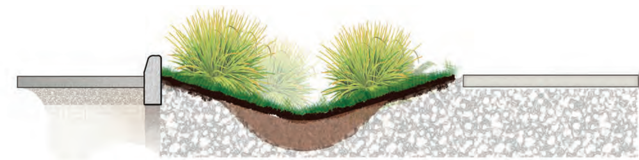
Figure 1: Rain Garden Section
