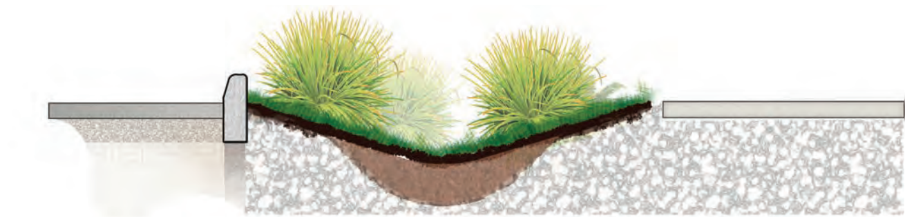
Figure 1: Rain Garden Section
