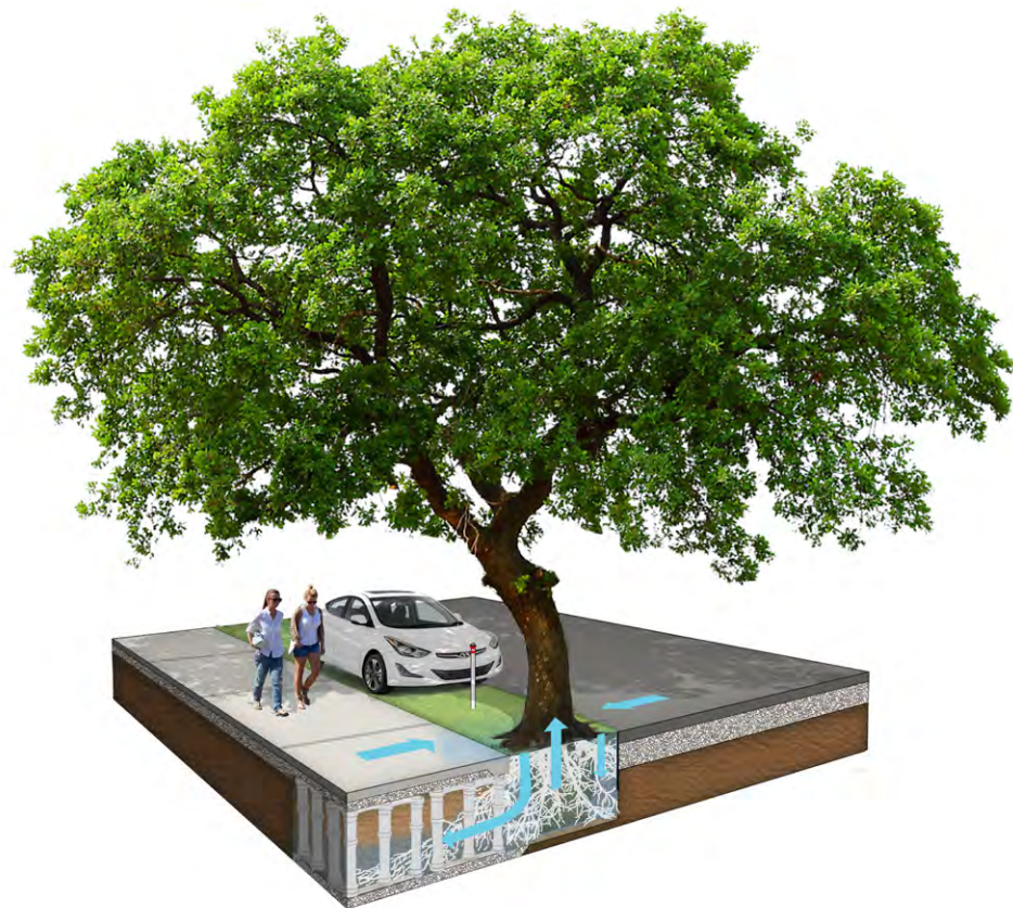
Large species tree in small swale - with Soil Cells
