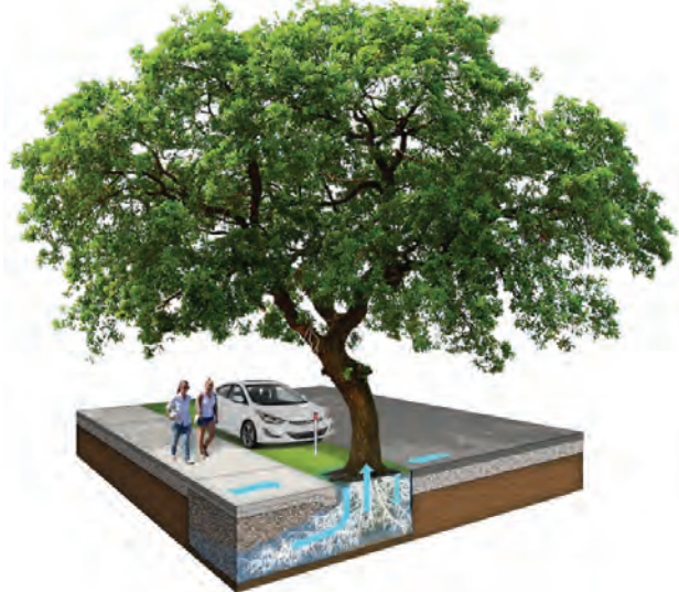
Illustration of a tree with Structural soil
