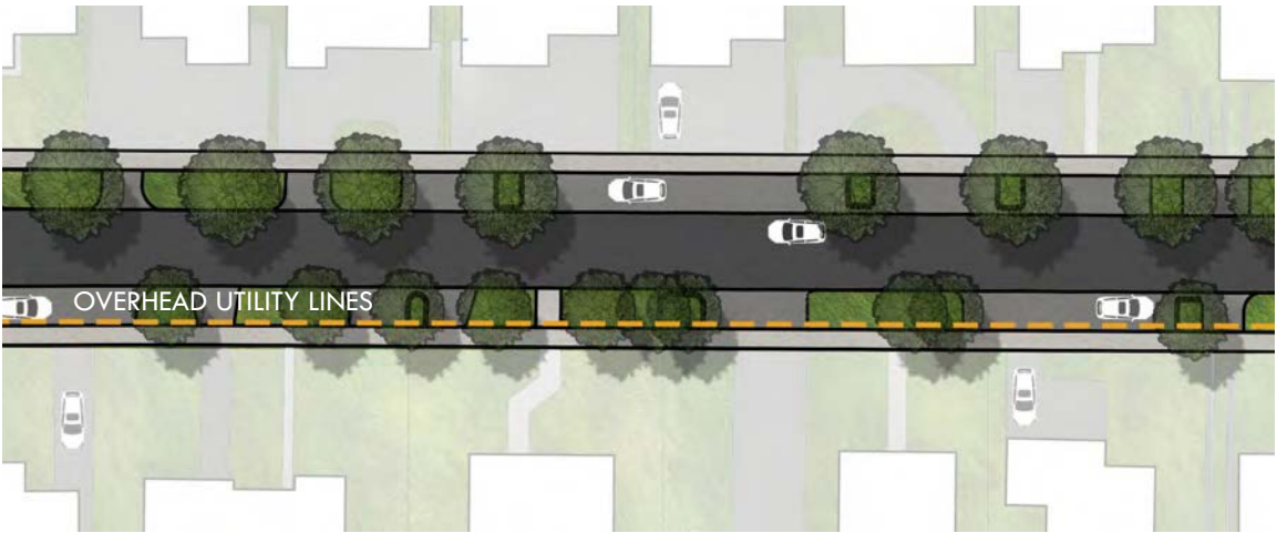
OVERHEAD UTILITY LINES ON ONE SIDE OF R.O.W
