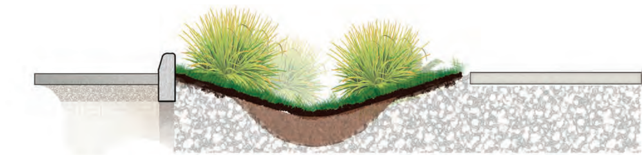
Figure 1: Rain Garden Section
